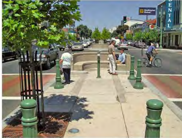
Pedestrian Median w/ Bollards & Street Furniture
