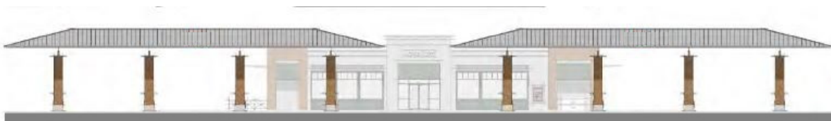
Figure 8-3. Roof Style – Hip Roof Canopy – ALLOWED
