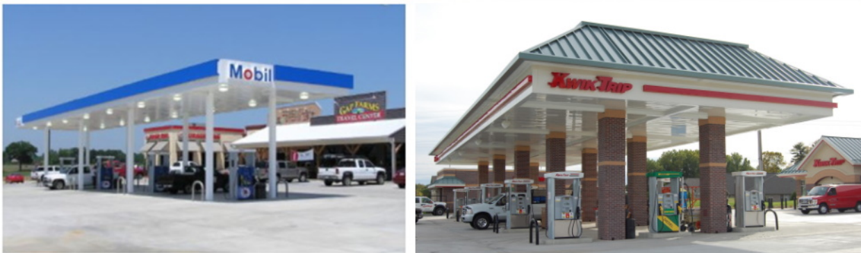
Figure 8-1. Roof Style - Flat Roofs greater than 24" in Height and Mansard Roofs – NOT ALLOWED.
