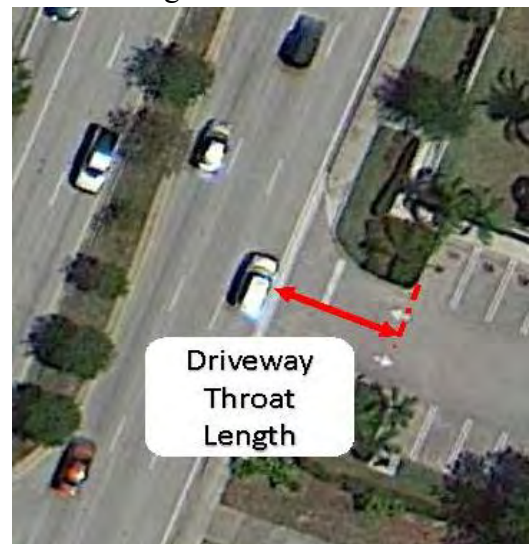
Figure 8-1 Driveway Throat Length
