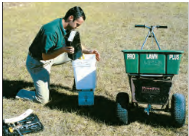
Figure 18. Weigh fertilizer to get accurate results.
