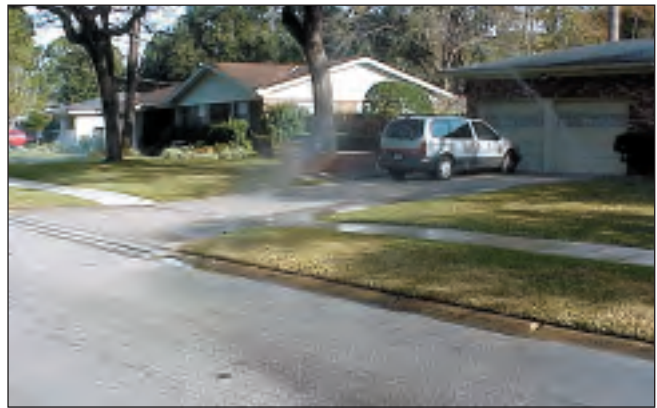
Figure 9. Overirrigation, runoff. Small turf area should be irrigated with spray heads, not sprinklers.
