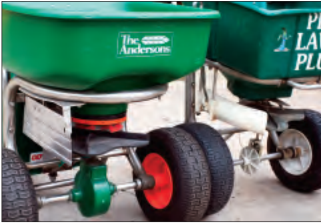
Figure 21. Spreaders with deflector shields.
